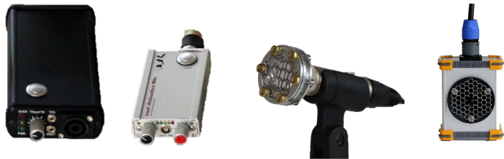
Figure 3: UltraSoundGate 116hm recording system: a. UltraSoundGate 116 player, b. UltraSoundGate 116hm recorder, c. CM16/CMP microphone, d. Ultrasonic Dynamic Speaker Vifa speaker.
